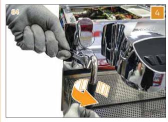
5 Utilizing a 24 mm wrench and a 20 mm one, block the front fitting and unscrew the copper pipe.
