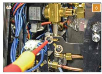
7 Extract the valves from the upper side and disconnect the cables.
