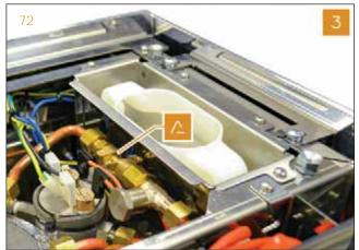
4 Utilizing a 14 mm and 17 mm wrenches, remove the incoming copper pipe from the boiler.
