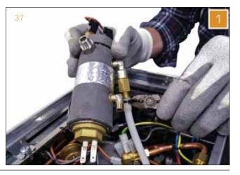
2 Utilizing a 14 mm wrench and a plier, remove the valve.
