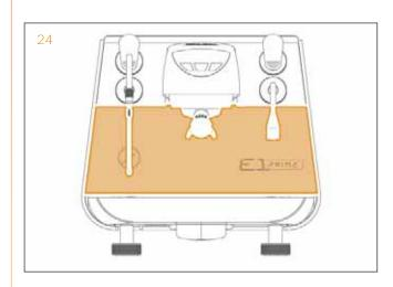
1 Remove the cup holder surface and both side panels .
