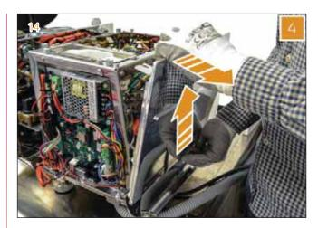
5 Disconnect the LED bar before to completely remove the panel.
