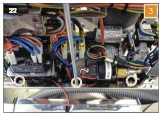
4 Using a 3 mm Allen Key, loosen the three screws to disassemble the panel.
