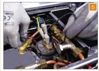
6 Utilizing a 12 mm and 13 mm wrenches, remove the temperature probe.
