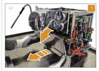
2 Utilizing a 3 mm Allen Key, partially unscrew the two screws holding the group cover.
