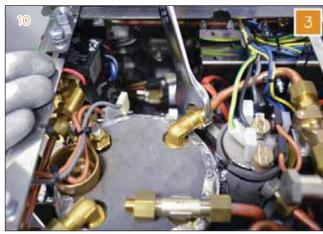
4 Utilizing a 17 mm wrench, disconnect the safety valve pipe.
