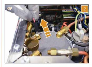
3 Utilizing a 17 mm wrench, disconnect the outlet steam pipe.
