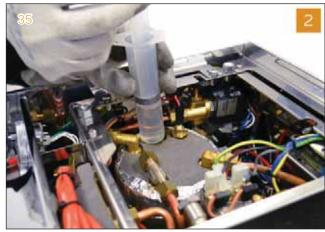
3 Utilizing a 13 mm wrench, disconnect the outgoing pipe from the auto-fill valve.
