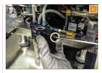
7 Place a cloth or absorbent paper underneath the valve and, utilising a 3 mm Allen key, remove the two screws that fix the body to the group.
