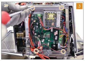
4 Remove the control unit support and, if preferred, disconnect the cables to simplify the operations.
