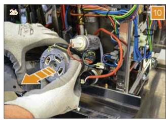
Once the pump-motor assembly has been removed, to replace the pump proceed as it follows:
