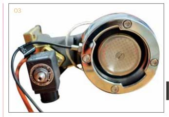
The shower is the interface between the coffee and the machine, preventing the coffee from rising inside the machine.
