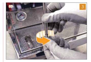
4 Utilizing a 9 mm wrench, block the upper part of the wand and, by hand, unscrew the middle part of the nozzle.
