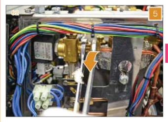
6 Utilizing a Philips screwdriver, remove the two screws that keep the hot water valve.
