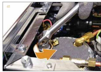
The steam safety valve is made to open at the pressure of 3 bar.
