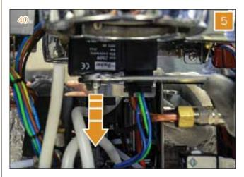
6 Utilizing a Philips screwdriver, remove the head screw.
