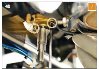
8 Remove the body of the valve. Check the contact points that often can be full of limescale. Clean utilising an adequately pointed tool.
