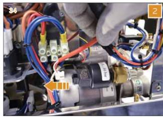
3 Unscrew and remove the pressure transducer by hand.
