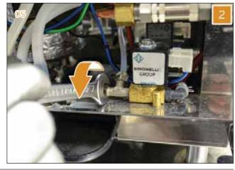
3 Disconnect the cables from the tank valve.
