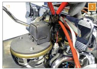
4 Utilizing a 13 mm wrench, loosen the sensor fixing nut.
