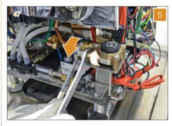
6 Utilizing a small Philips screwdriver, remove the two screws that keep the flowmeter on the bracket.
