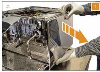
2 Remove the work surface pulling out the drip tray.
