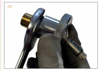
9 The junction is visible now, with its spring. Notice that there is a white Teflon o-ring inside the joint.
