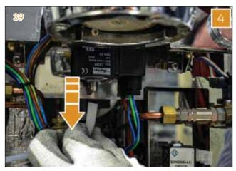
5 Utilizing a 14 mm wrench, unscrew the fixing nut of the coil.
