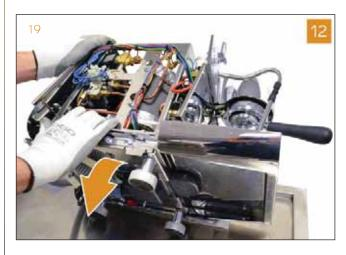
13 Utilizing a 10 mm wrench, remove the two nuts.
