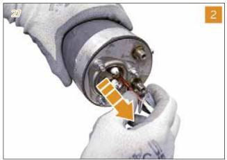
3 Utilizing a 10 mm wrench, remove the three nuts.
