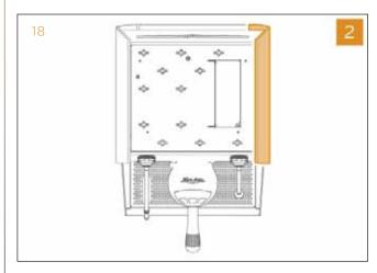
3 Rotate the machine on the right side, being careful to not damage it.
