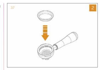
3 Place the manufacturer's recommended dose of specific powder detergent inside and put the filter holder into the group.
