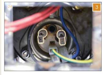
4 Utilizing a tester, check the heating element (value 34 ± 2 Ohm).
