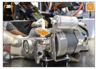
13 Utilizing a 9 mm wrench, remove the T outgoing fitting of the pump.
