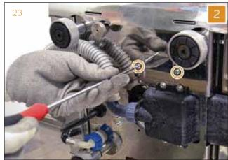
3 Disconnect the electrical resistance cables. For easier access, it is useful to remove the safety thermo-fuse too.
