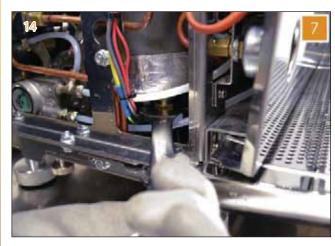
8 Utilizing a 17 mm wrench, disconnect the inlet pipe.
