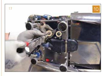
11 Disconnect the five electrical cables, corresponding to: thermal fuse, heating element and mass.
