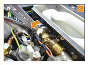
5 Utilizing a 13 mm and 17 mm wrenches, keep the T connection and remove the outgoing copper pipe.
