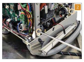
3 Utilizing a Philips screwdriver, loosen the three screws on the bottom.
