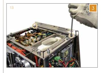
4 With a hand pull the high side of the panel and with the other hand lift it from the bottom.
