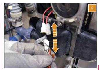
5 Utilizing a tester, check the continuity of the safety thermo-fuse.
