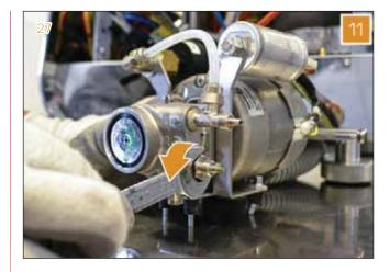
12 Utilizing a 12 mm wrench, remove the Teflon pipe.
