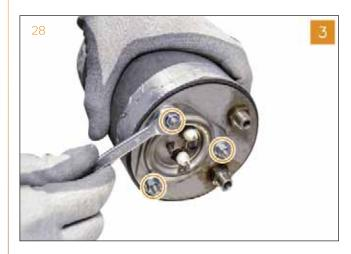
4 With the help of a screwdriver, remove the heating element.
