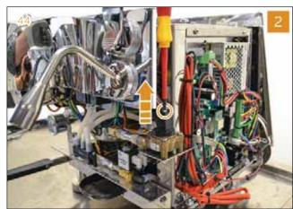
3 Utilizing a 14 mm and 17 mm wrenches, remove the outgoing pipe from the flowmeter.
