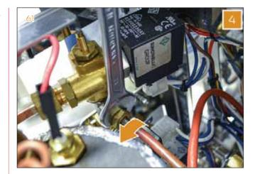
5 Utilizing two 17 mm wrenches, remove the inlet pipe from the cold water valve.
