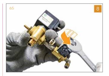
9 Utilizing a 14 mm wrench, unscrew the valve base.
