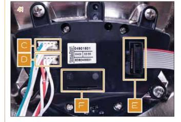
The DIP switch is accessible by removing its small cover (F). Its setting permits to the control unit to correctly identify the service board.
