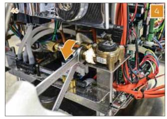
5 Utilizing two 17 mm wrenches, remove the inlet pipe from the flowmeter.
