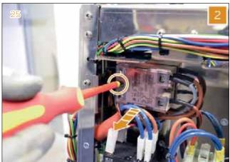
3 Utilizing a Philips screwdriver, loosen the four screws and remove the cables.
