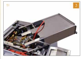
4 Utilizing a 5,5 mm wrench, remove the four nuts fixing the sensor cover and open it.
