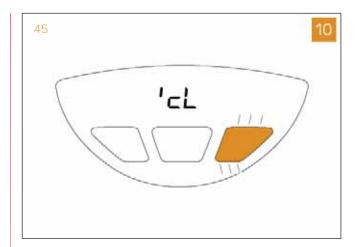
11 Once the washing phase is complete, the machine stops and the **IC** button remains ON.
