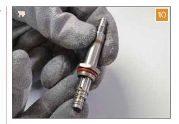
11 If the replacement of the valve body is necessary, utilize a 14 mm and 16 mm wrenches to disassemble the valve.
