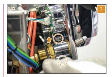
8 Utilizing a 24 mm wrench or simply by hand, remove the fitting.
