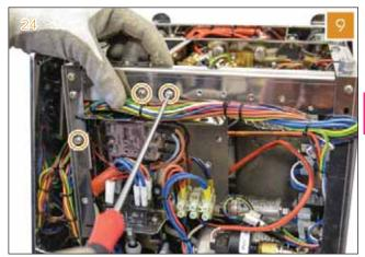
9 Remove the static relay bracket.
