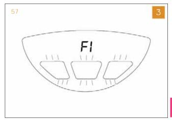
4 Press and hold the **IA** and **IC** buttons together until procedure is engaged (the pump starts to run).
