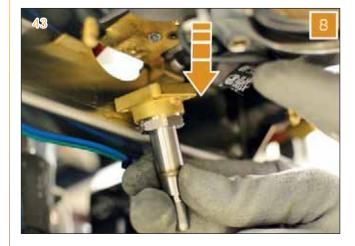
9 Utilizing a vise and a 24 mm wrench, unscrew the valve base and check for the presence of limescale or oily residues.
