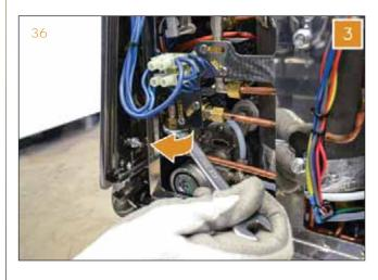
4 Utilizing a 13 mm and a 12 mm wrenches, disconnect the inlet pipe from the auto-fill valve.
