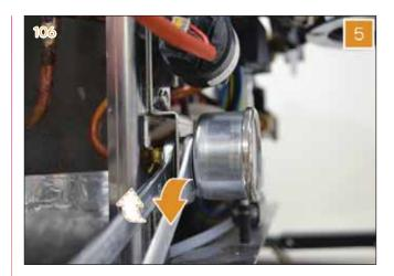
6 Utilizing a 13 mm wrench, keep the nut and loosen the pressure gauge by hand.
