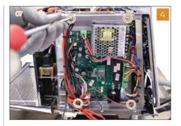
5 Remove the control unit support and, if preferred, disconnect the cables to simplify the operations.
