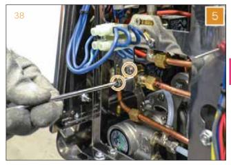
6 Extract the auto-fill valve from the upper side and disconnect the cables.
