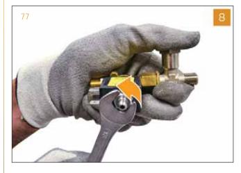
9 Utilizing a vise and a 16 mm wrench, unscrew the valve base.
