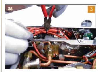
4 Following the orange cable, disconnect the heating element from the neutral and from the high-limit thermostat.
