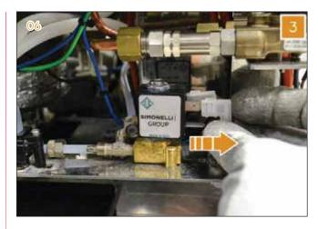
4 Utilizing a small screwdriver, unscrew the two screws that fix the valve to the frame.
