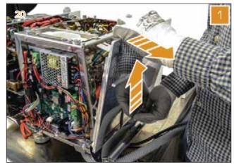
2 Utilizing a Philips screwdriver, remove the two lateral screws.
