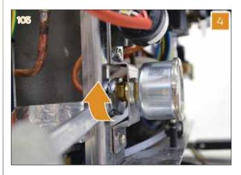
5 Utilizing a 12 mm and a 13 mm wrenches, block the pressure gauge and loosen the nut.
