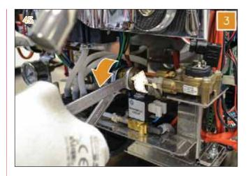
4 Utilizing a 12 mm and 13 mm wrenches, remove the not return valve.
