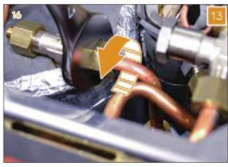
14 Utilizing a 17 mm wrench and keeping the coffee boiler, unscrew the outlet pipe to the group.
