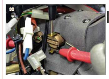
• If there is not continuity, rearm the high-limit thermostat pushing into the hole (A) by a small screwdriver.
