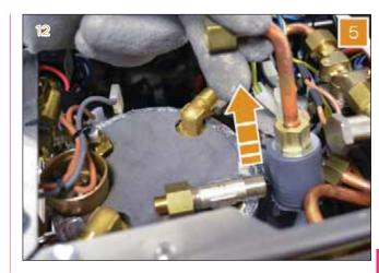
6 Utilizing a 17 mm wrench, disconnect the pressure sensor pipe.
