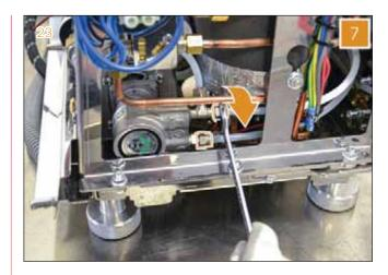
8 Utilizing a Philips screwdriver, remove the three screws that fix the static relay bracket.
