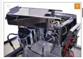
10 Disconnect the two heating element cables from the bottom of the coffee boiler.
