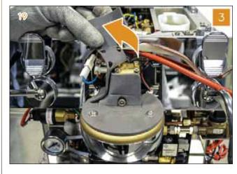
4 Utilizing a 3 mm Allen key, remove the four screws and open the chamber.
