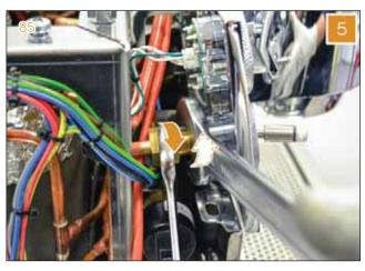
6 Utilizing a 24 mm wrench, loosen the fitting.
