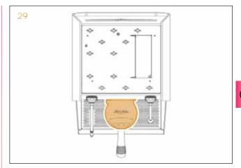
1 Remove the side panels, the drip tray and the lower front panel, as described in the previous paragraphs.
