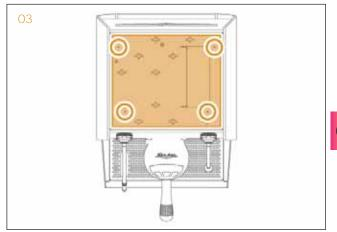
1 Utilising a Philips screwdriver, remove the 4 screws of the module.
