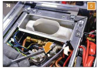
6 Extract the valve and disconnect the cables.
