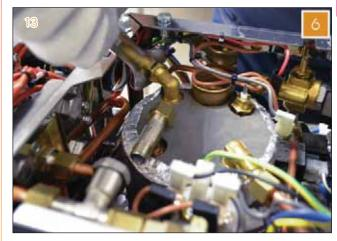
7 Utilizing a 17 mm wrench, disconnect the hot water pipe.
