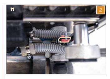
3 Remove the cup holder surface. The steam valve (A) is located on the right side, between the tank and the coffee boiler.
