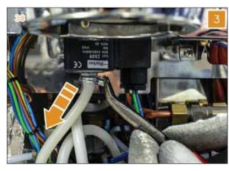
4 Disconnect the Teflon pipe of the third outlet.
