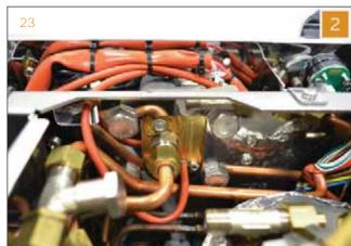
3 Following the orange cable, cut the clamps to release the cable.
