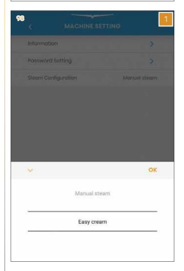
2 Utilizing the Victoria Arduino El App, in the programming of the MYCOFFEE recipe, set the Easycream parameters and save.
