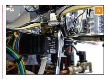
5 Utilizing an adjustable wrench, slide out the sensor.
