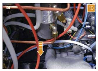
11 Utilizing a 13 mm wrench by entering from the right side of the machine, and keeping the coffee boiler with the other hand, unscrew the inlet coffee boiler pipe.
