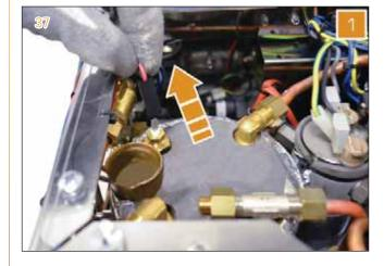
2 Utilizing a 17 mm cup hex wrench, unscrew the probe from its housing.
