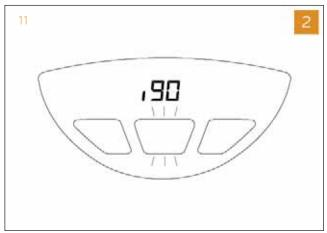
3 Press the **1A** and **1C** buttons to decrease or increase the temperature. Display will show the set temperature.
