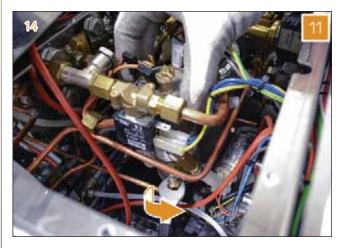
12 Reposition the water tank support.
