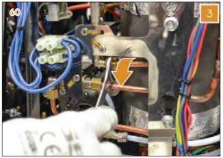
4 Utilizing a 13 mm wrench, remove the outgoing pipe from the hot and cold water valves.
